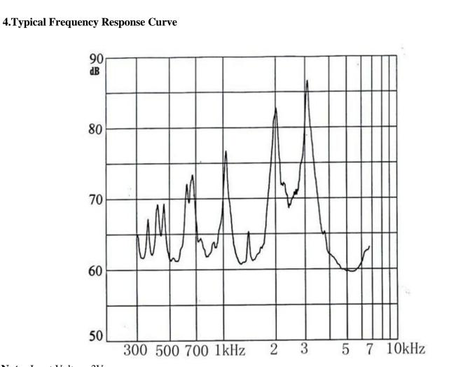
**Note:** Input Voltage 3Vp-p square wave Distance 10 cm
